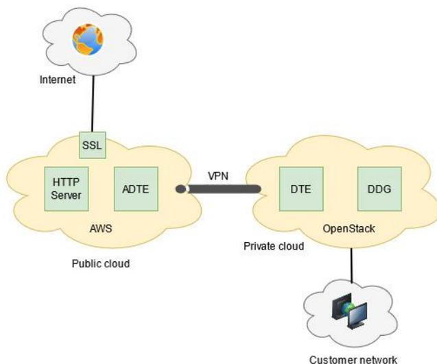
**Figure 6: Architecture of the deployed system.**
