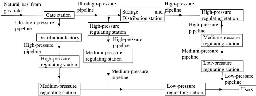
**Figure 1: Schematic diagram of urban natural gas pipeline network system.**
