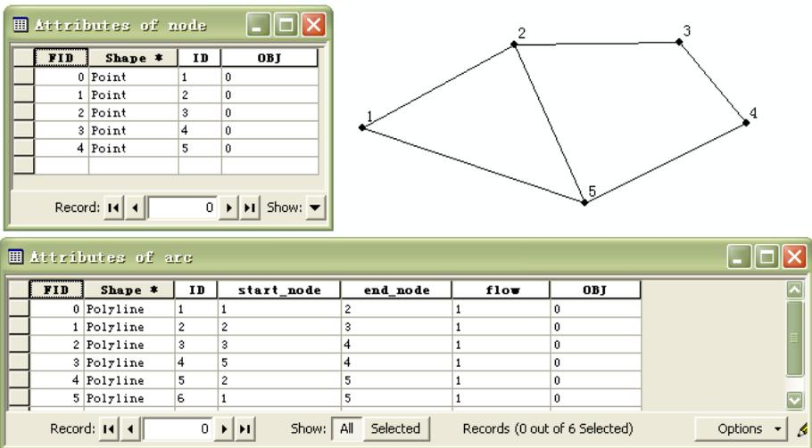
**Figure 2: Schematic diagram of the recording of attributes of points and lines in a virtual network.**
