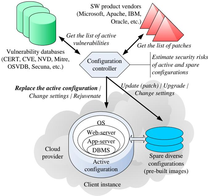
Figure 1. General architecture of the cloud-based intrusion-avoidance deployment environment.
