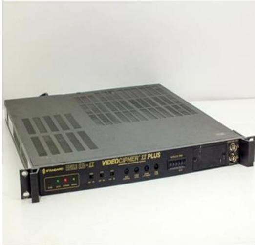
**Figure 2: Video Cipher scrambler device analog content protection for TV operators.**
